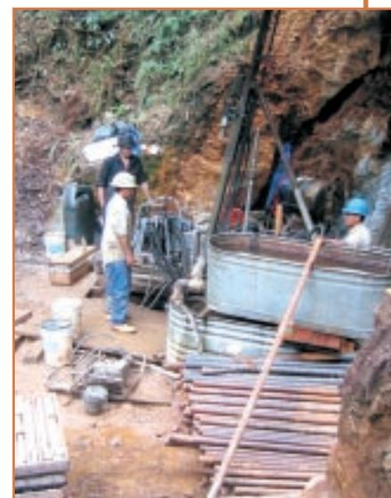
*Drilling with portable rig at Mirador*
