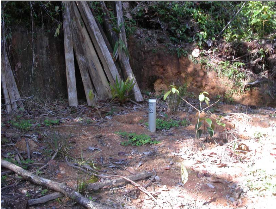
Figure 11.2 Drill hole Collar Marker
