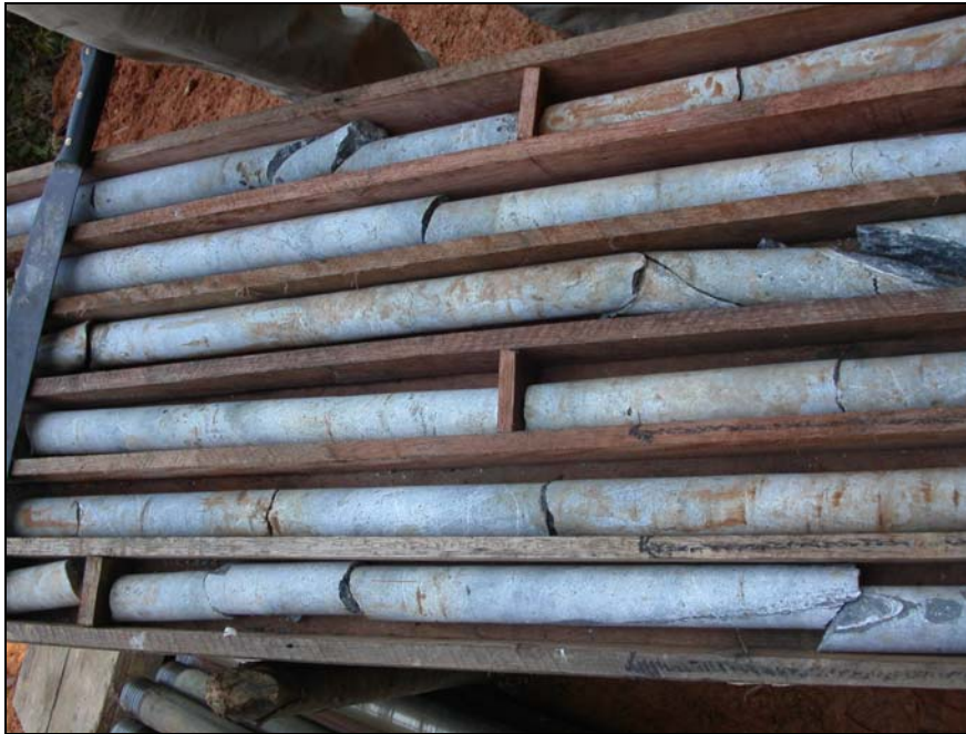
Figure 7.3 Drill Core with Unaltered Anhydrite (Below the Gypsum Front)
