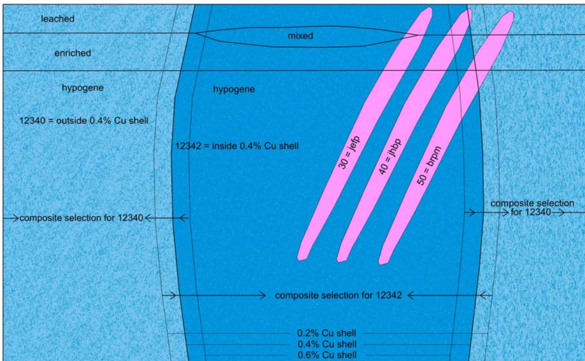
Figure 17.2 Schematic Illustration of Rock and Mineral Zones Used for Estimation - Gold and Silver
